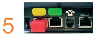
**5** **On the last Remote Terminal, plug the RED loopback into the YELLOW port to close the circuit.**
